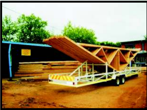
Pre Fabricates Roof Trusses
